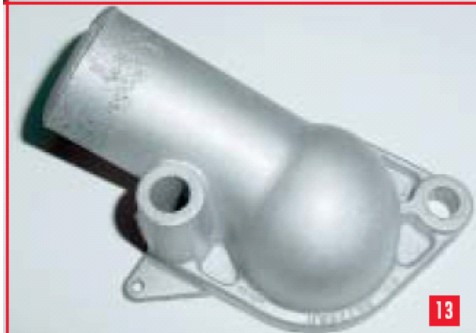
13 Here’s “the house” where your thermostat dwells. “Shoot” it with an I.R. gun to determine your engine’s actual operating temperature, and compare that with the temperature gauge so you know what the gauge is telling you.
