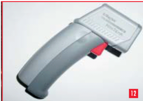
12 The Raytek MiniTemp MT-4 infrared temperature gun, the best cooling system diagnostic tool you can buy. It tells you the exact temperature of any component the red laser dot is aimed at.
